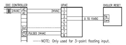
The UPAC/ADJ is configured for PWM or FLT input by selecting the appropriate dip switch setting. The UPAC adjustable outputs are 0-5VDC thru 0-15VDC. In this application the 1-15VDC output is used to reset a chiller. Zero and V span adjustment potentiometers allow for field calibration of the voltage output. See FIELD SETUP AND CALIBRATION section for dip switch settings and calibration.
