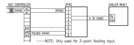
The UPAC/STD is configured for PWM or FLT input by selecting the appropriate DIP switch setting. The UPAC standard outputs are 0-10VDC and 4-20mA. In this application the 0-10VDC output is used to reset a chiller. Zero and span adjustment potentiometer allow for field calibration of the 4-20mA output. See FIELD SETUP AND CALIBRATION section for dip switch settings and calibration.
