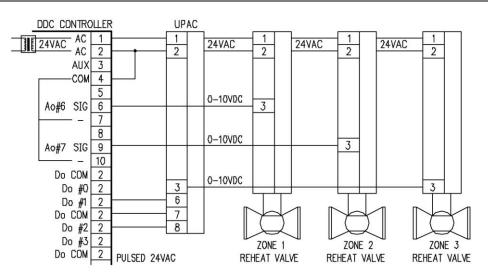
The UPAC/STD is configured for PWM or FLT input by selecting the appropriate DIP switch setting. The UPAC standard outputs are 0-10VDC and 4-20mA. In this application the UPAC's 0-10VDC output is used to drive a third STAEFA's 599 MZ valve actuator.
