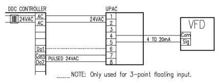
The UPAC/STD is configured for PWM or FLT input by selecting the appropriate DIP switch setting. The UPAC standard outputs are 0-10VDC and 4-20mA. In this application the 4-20mA output is used to drive a VFD. Zero and span adjustment potentiometer allow for field calibration of the 4-20mA output. See FIELD SETUP AND CALIBRATION section for dip switch settings and calibration.
