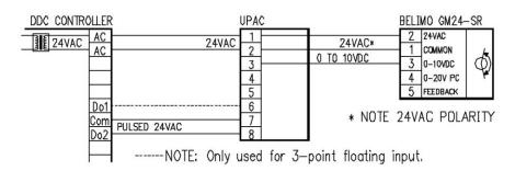
The UPAC/STD is configured for PWM or FLT input by selecting the appropriate DIP switch setting. The UPAC standard outputs are 0-10VDC and 4-20mA. In this application the UPAC's 0-10VDC output is used to drive a Belimo actuator. Zero and span adjustment potentiometer allow for field calibration of the 4-20mA output. See FIELD SETUP AND CALIBRATION section for dip switch settings and calibration.
